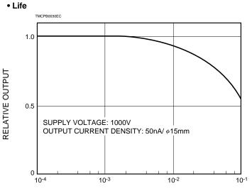
ACCUMULATED CHARGE OF OUTPUT SIGNAL (C / cm<sup>2</sup>)
