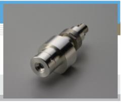
B749 is a photon drag detector that utilizes the photon drag effect in which carriers created by input photons are dragged in the direction of photons, generating an electromotive force. B749 ensures high-speed operation even at room temperatures and has high sensitivity in the 10 µm band, making it well suited to detection of CO<sub>2</sub> lasers. An easy-to-use detector module integrated with a preamplifier (B7506-01) is also available.
