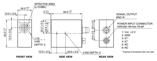
Power cable with connector (HIROSE HR10A-7P-6S) is supplied with H7828 series
