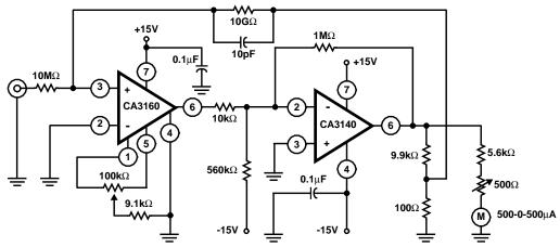
FIGURE 11. CURRENT-TO-VOLTAGE CONVERTER TO PROVIDE A PICOAMMETER WITH ±3pA FULL SCALE DEFLECTION
