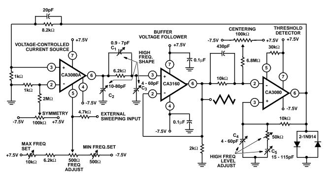
FIGURE 9A. 1,000,000/1 SINGLE CONTROL FUNCTION GENERATOR: 1Hz to 1MHz
