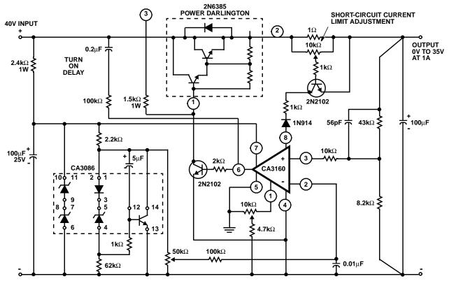
Hum and Noise Output <250µV<sub>RMS</sub>; Regulation (No Load to Full Load) <0.005%; Input Regulation <0.01%/V
