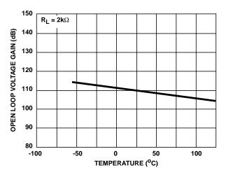
FIGURE 16. OPEN LOOP GAIN vs TEMPERATURE
