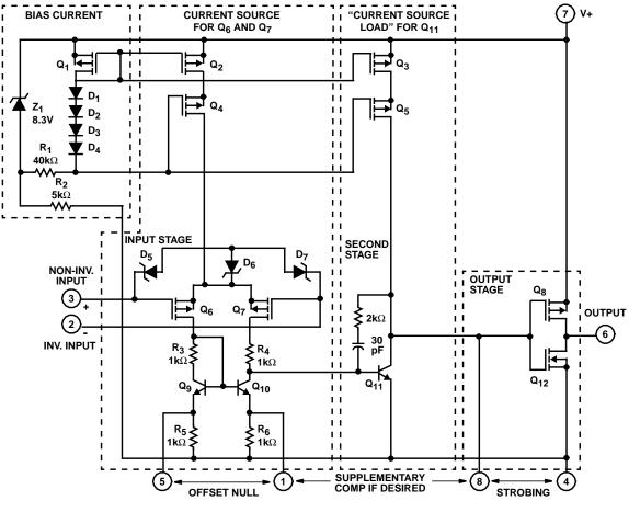
NOTE: Diodes D5 Through D7 Provide Gate Oxide Protection For MOSFET Input Stage.
