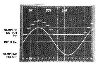
Top Trace: Sampled Output Center Trace: Input Signal Bottom Trace: Sampling Pulses
