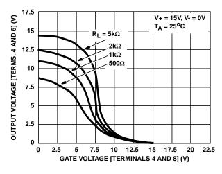
FIGURE 17. VOLTAGE TRANSFER CHARACTERISTICS OF CMOS OUTPUT STAGE
