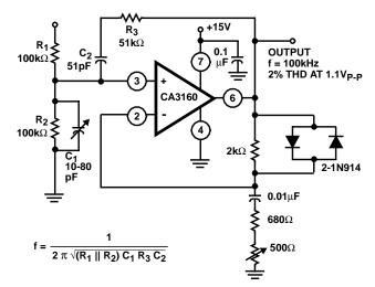
FIGURE 13. SINGLE SUPPLY WEIN BRIDGE OSCILLATOR
