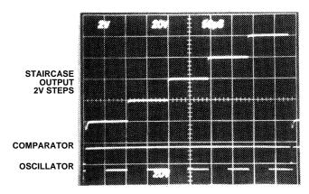
Top Trace: Staircase Output 2V Steps Center Trace: Comparator Bottom Trace: Oscillator
