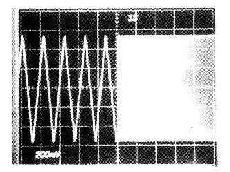
NOTE: A square wave signal modulates the external sweeping input to produce 1Hz and 1MHz, showing the 1,000,000/1 frequency range of the Function Generator.
