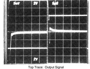
Center Trace: Difference Signal 5mV/Div. Bottom Trace: Input Signal FIGURE 3C. INPUT-OUTPUT DIFFERENCE SIGNAL SHOWING
