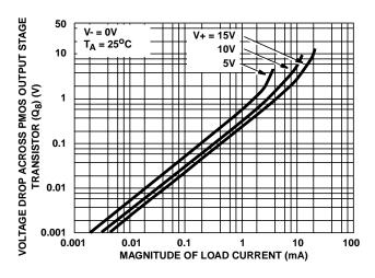
FIGURE 20. VOLTAGE ACROSS PMOS OUTPUT TRANSISTOR (Q8) vs LOAD CURRENT
