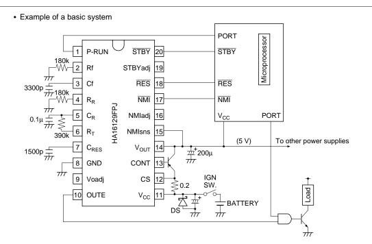
· Example of a system using a backup circuit and a primary voltage monitoring circuit
