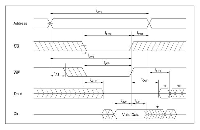
Write Timing Waveform (2) (OE Low Fixed)
