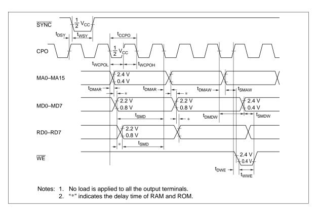
HD61830 LCD Driver Interface (V  $_{CC}$  = 5 V  $\pm 10\%,\,GND$  = 0 V,  $T_a$  = –20 to +75°C)
