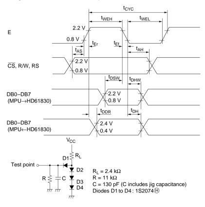
HD61830 External RAM and ROM Interface ( $V_{CC}$  = 5 V ±10%, GND = 0 V,  $T_a$  = -20 to +75°C)
