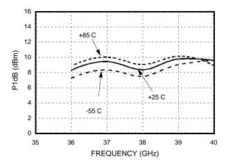
All data is with the chip in a 50 ohm test fixture connected via ribbon bonds of minimal length.
