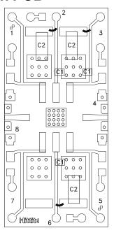
The grounded Co-Planar Wave Guide (G-CPW) PCB input/output transitions allows use of Ground-Signal-Ground (GSG) probes for testing. Suggested probe pitch is  $400\mu m$  (16 mils). Alternatively, the board can be mounted in a metal housing with 2.4 mm coaxial connectors.
