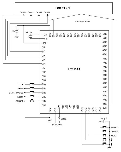
Note: The IC substrate should be connected to VSS in the PCB layout artwork.
