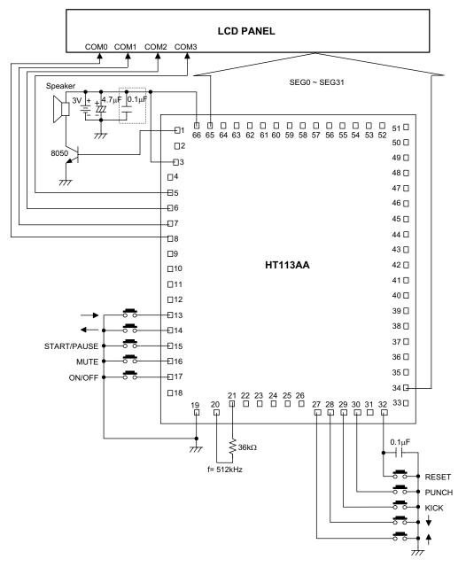
Note: The capacitor in dash block is recommended.
