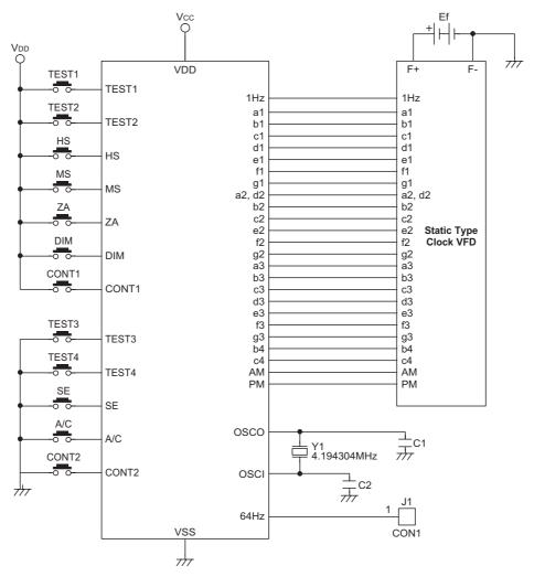
Note: Capacitors C1 and C2 can adjust the frequency accuracy
