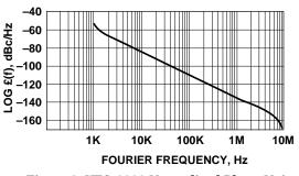
Figure 2. VTO-9032 Normalized Phase Noise @ 640 MHz S.S.B. Power Spectral Density.
