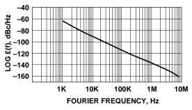
Figure 4. VTO-9050 Normalized Phase Noise @ 1000 MHz S.S.B. Power Spectral Density.
