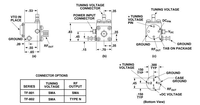
Figure 13. TO-8 Test Fixture.
