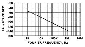
Figure 8. VTO-9090 Noise @ 1000 MHz Single Sideband Phase Noise.
