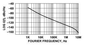
Figure 10. VTO-9120 Normalized Phase Noise @ 2000 MHz S.S.B. Power Spectral Density.
