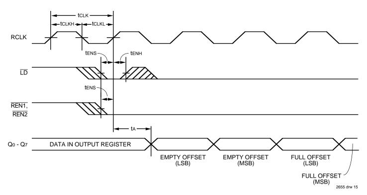
Figure 13. Read Offset Registers Timing
