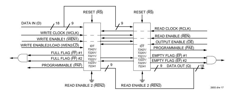
Figure 15. Block Diagram of 64 x 18/256 x 18/512 x 18/1024 x 18/2048 x 18/4096 x 18 Synchronous FIFO Used in a Width Expansion Configuration
