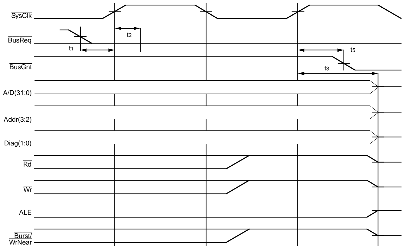
Figure 16. Request and Relinquish of R3081 Bus to External Master
