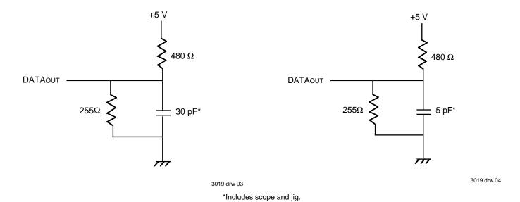
Figure 1. Output Load
