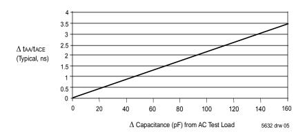
Figure 3. Typical Output Derating (Lumped Capacitive Load).
