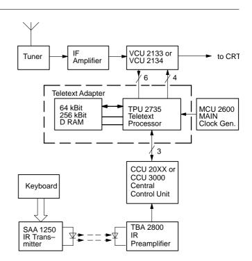
Fig. 1–1: Teletext application block diagram
