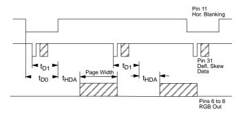
Fig. 7-4: Horizontal display start in double-scan mode
