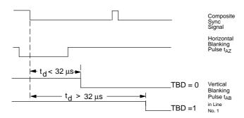
Fig. 7-1: Timing diagram for the horizontal and vertical blanking pulses  $t_{\text{AZ}}$  and  $t_{\text{AB}}$  for two cases
