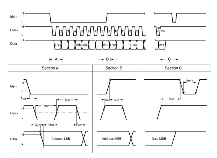
Fig. 12-1: IM bus waveforms
