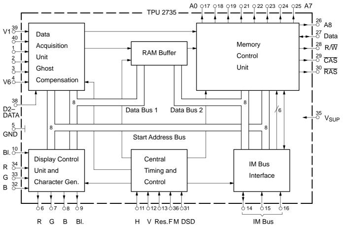
Fig. 2-1: Block diagram of the TPU 2735
