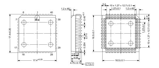
Fig. 3–2: TPU 2735 in 44-pin PLCC package, Weight approx. 2.2 g, Dimensions in mm
