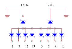
The EiMDXXC8 is designed to provide transient suppression on multiple data lines and I/O ports. The low profile SO-14 design allows the user to protect up to eight data and I/O lines with one package. The bidirectional device and may be used on lines where the normal operating voltage is above and below ground (i.e. +12V to -12V). The EiMDXXC8 TVS diode network will meet the surge requirements of IEC 1000-4-2, Level 4, "Human Body Model" for air and contact discharge.
