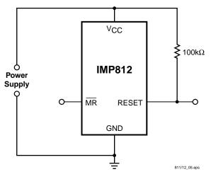
Figure 3. RESET Valid with V<sub>CC</sub> Under 1.1V
