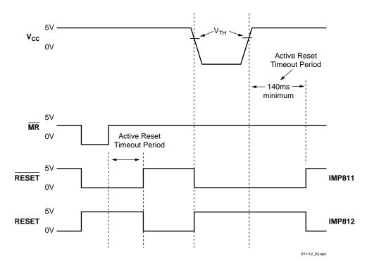
Figure 1. Reset Timing and Manual Reset (MR)
