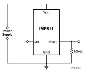
Figure 2. RESET Valid with V<sub>CC</sub> Under 1.1V
