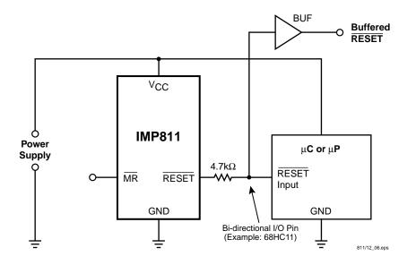
Figure 4. Bi-directional Reset Pin Interface
