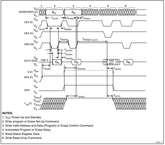
Figure 17. AC Waveforms for Write Operations (WE#–Controlled Writes) SEE NEW DESIGN RECOMMENDATIONS
