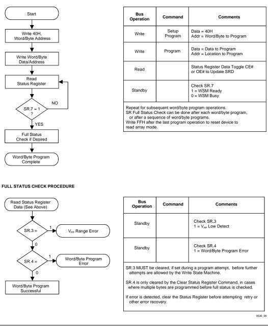
Figure 9. Automated Word/Byte Programming Flowchart
