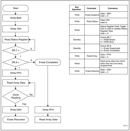
Figure 11. Erase Suspend/Resume Flowchart
