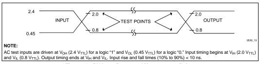
Figure 20. 5 V Input Range and Measurement Points
