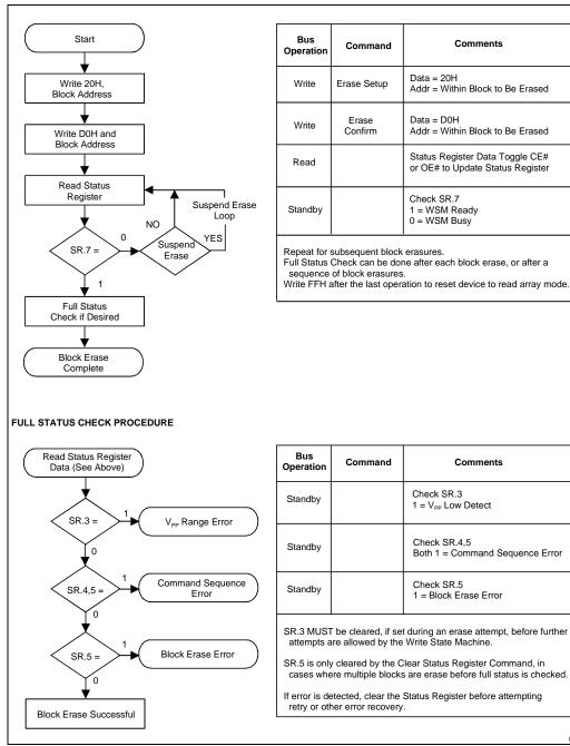
Figure 10. Automated Block Erase Flowchart
