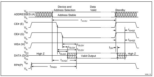
Figure 15. AC Waveforms for Read Operations
