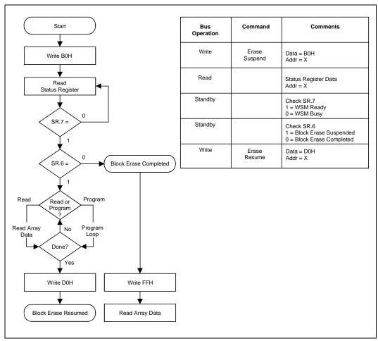
Figure 9. Block Erase Suspend/Resume Flowchart
