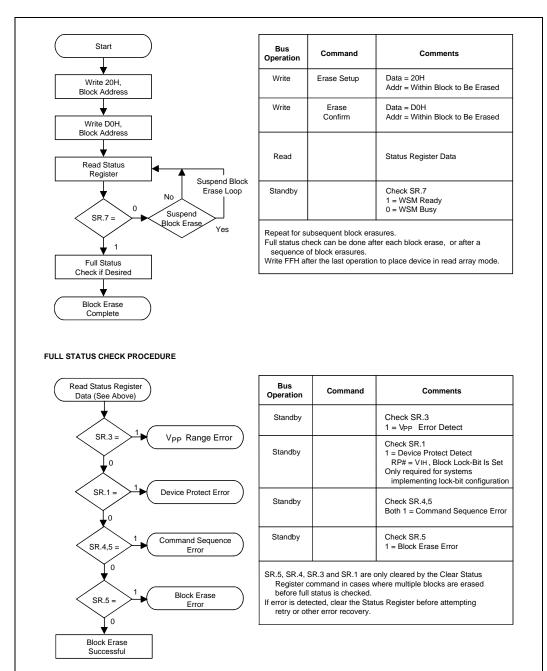
Figure 7. Automated Block Erase Flowchart
