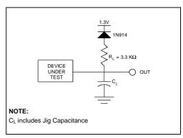
Figure 16. Transient Equivalent Testing Load Circuit
