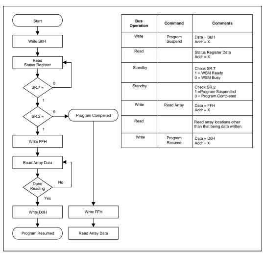
Figure 10. Program Suspend/Resume Flowchart
