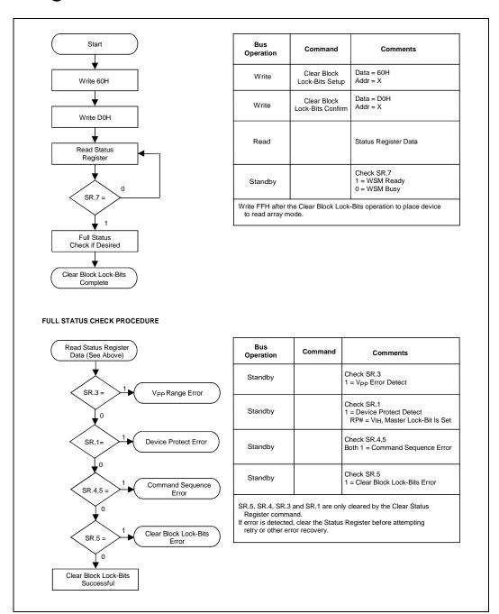
Figure 12. Clear Block Lock-Bits Flowchart
