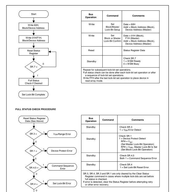
Figure 11. Set Block and Master Lock-Bit Flowchart
