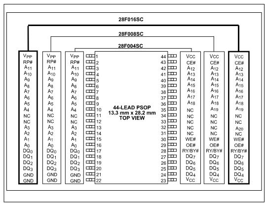
Figure 3. PSOP 44-Lead Pinout
