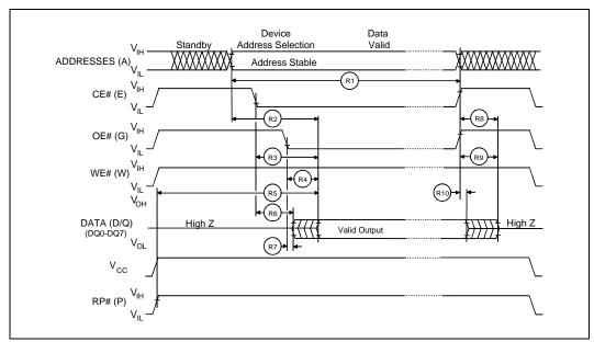
Figure 18. AC Waveform for Read Operations
