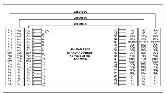
Figure 2. TSOP 40-Lead Pinout
