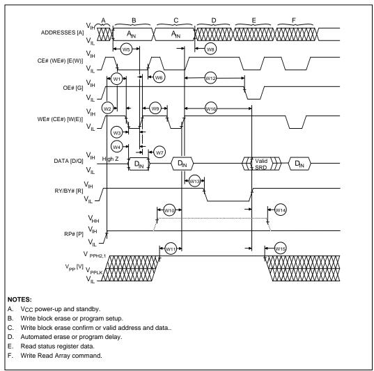
Figure 19. AC Waveform for Write Operations
