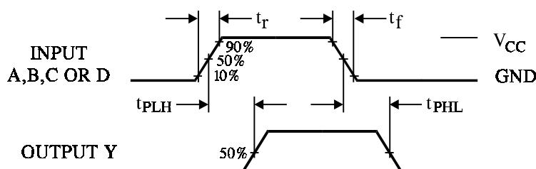
Figure 1. Switching Waveforms
