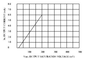
Figure 3. Output Sink Current versus Output Saturation Voltage
