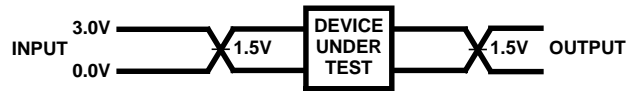
NOTE: AC Testing: Inputs are driven at 3.0V for Logic "1" and 0.0V for Logic "0". Input and output timing measurements are made at 1.5 for both a Logic "1" and "0". CLK is driven at 4.0 and 0V and measured at 2.0V. FIGURE 13. AC TESTING INPUT, OUTPUT WAVEFORM
