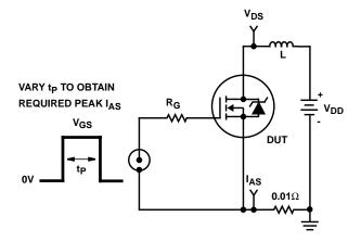
FIGURE 12. UNCLAMPED ENERGY TEST CIRCUIT
