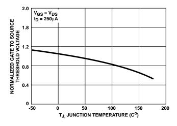
FIGURE 8. NORMALIZED GATE THRESHOLD VOLTAGE vs JUNCTION TEMPERATURE
