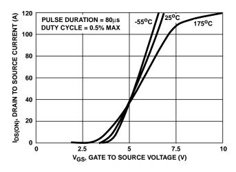
FIGURE 6. TRANSFER CHARACTERISTICS
