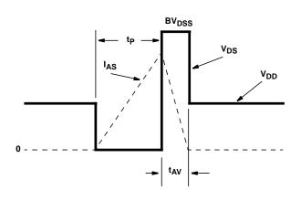
FIGURE 13. UNCLAMPED ENERGY WAVEFORMS
