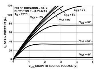
FIGURE 5. SATURATION CHARACTERISTICS
