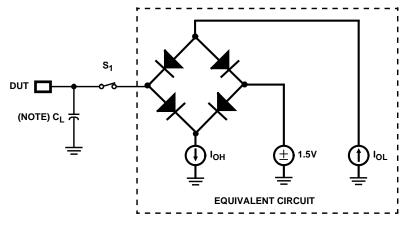
SWITCH  $\text{S}_{1}$  OPEN FOR  $\text{I}_{\text{CCSB}}$  AND  $\text{I}_{\text{CCOP}}$  TEST
