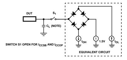
NOTE: Test head capacitance.
