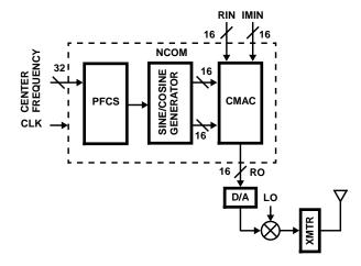
FIGURE 5. QUADRATURE AMPLITUDE MODULATION (QAM)
