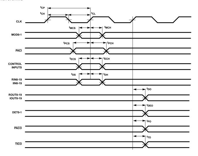
FIGURE 7. INPUT AND OUTPUT TIMING
