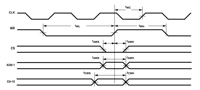
FIGURE 8. CONTROL BUS TIMING
