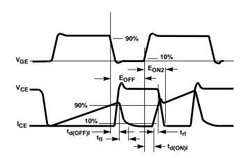
FIGURE 19. SWITCHING TEST WAVEFORMS
