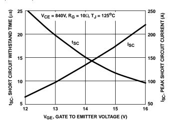
FIGURE 4. SHORT CIRCUIT WITHSTAND TIME
