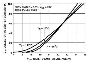
FIGURE 13. TRANSFER CHARACTERISTIC
