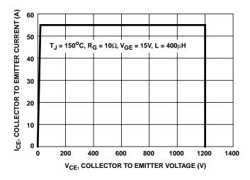
FIGURE 2. MINIMUM SWITCHING SAFE OPERATING AREA
