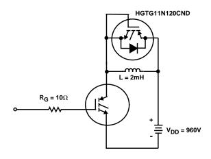
FIGURE 18. INDUCTIVE SWITCHING TEST CIRCUIT
