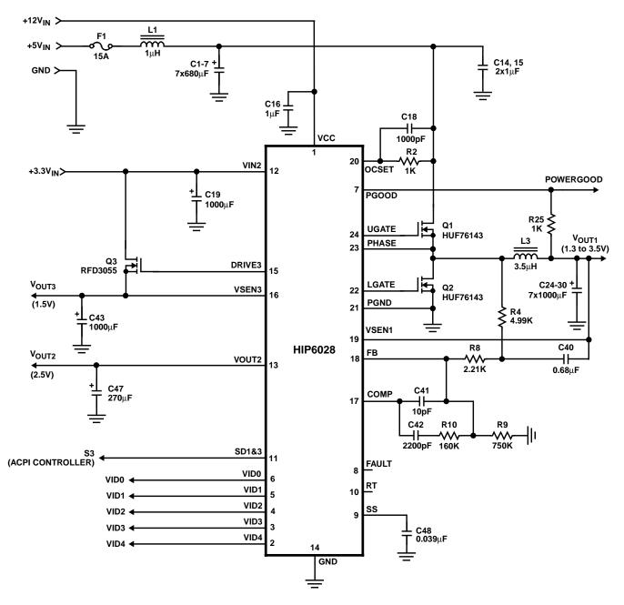
FIGURE 16. APPLICATION CIRCUIT
