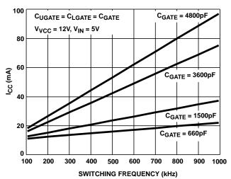
FIGURE 5. BIAS SUPPLY CURRENT vs FREQUENCY
