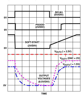
FIGURE 10. POWER-SAVING SHUTDOWN SEQUENCE DETAIL
