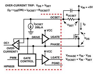
FIGURE 9. OVER-CURRENT DETECTION
