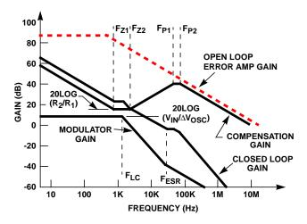
FIGURE 13. ASYMPTOTIC BODE PLOT OF CONVERTER GAIN
