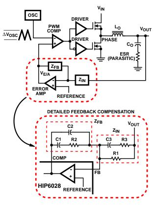
FIGURE 12. VOLTAGE-MODE BUCK CONVERTER COMPENSATION DESIGN
