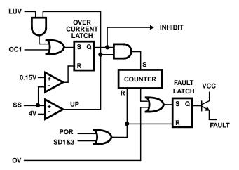
FIGURE 7. FAULT LOGIC - SIMPLIFIED SCHEMATIC
