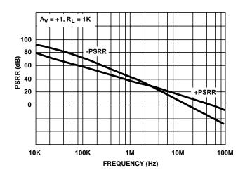
FIGURE 10. PSRR vs FREQUENCY
