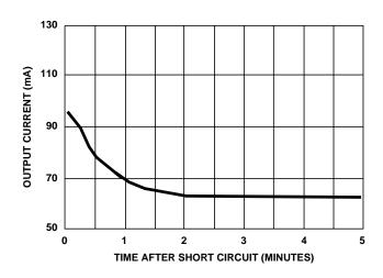
FIGURE 24. SHORT CIRCUIT OUTPUT CURRENT vs TIME
