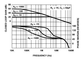
FIGURE 8. VARIOUS CLOSED LOOP GAINS vs FREQUENCY
