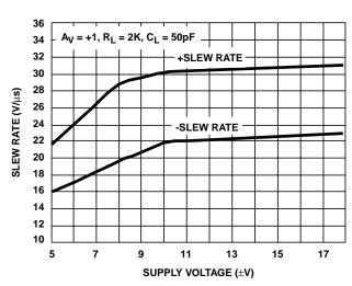
FIGURE 18. SLEW RATE vs SUPPLY VOLTAGE
