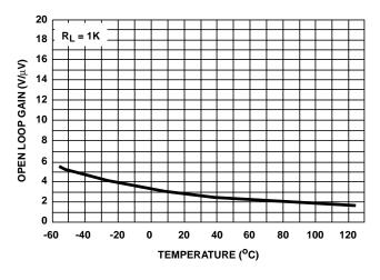
FIGURE 11. OPEN LOOP GAIN vs TEMPERATURE
