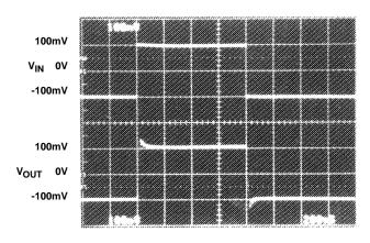
$V_{OUT} = \pm 100 \text{mV}$ Vertical Scale = 100 mV/Div., Horizontal Scale = 200 ns/Div.
