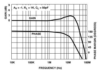
FIGURE 7. CLOSED LOOP GAIN vs FREQUENCY
