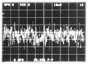
Vertical Scale = 10mV/Div.; Horizontal Scale = 1s/Div.  $A_V = +25,000; \, E_N = 1.5 \mu V_{P-P} \; RTI$
