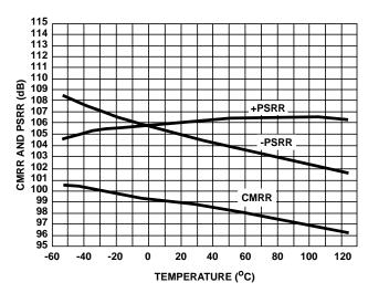
FIGURE 22. CMRR AND PSRR vs TEMPERATURE
