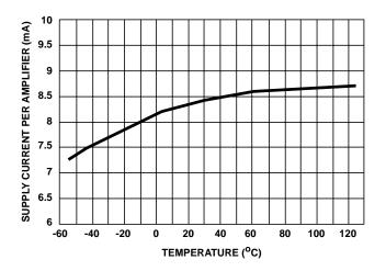
FIGURE 29. SUPPLY CURRENT/AMPLIFIER vs TEMPERATURE
