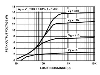
FIGURE 28. OUTPUT VOLTAGE SWING vs LOAD RESISTANCE
