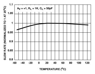
FIGURE 15. SLEW RATE vs TEMPERATURE
