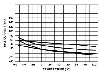
FIGURE 13. BIAS CURRENT vs TEMPERATURE (4 REPRESENTATIVE UNITS)
