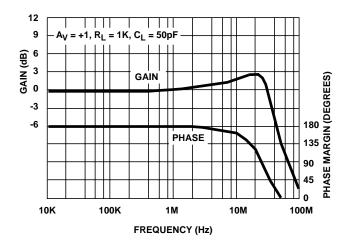
FIGURE 6. CLOSED LOOP GAIN vs FREQUENCY
