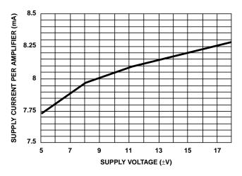
FIGURE 17. SUPPLY CURRENT vs SUPPLY VOLTAGE
