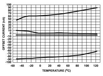
FIGURE 21. OFFSET CURRENT vs TEMPERATURE (4 REPRESENTATIVE UNITS)
