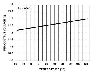
FIGURE 14. OUTPUT VOLTAGE SWING vs TEMPERATURE
