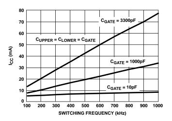
FIGURE 2. BIAS SUPPLY CURRENT vs FREQUENCY
