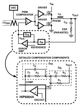
FIGURE 7. VOLTAGE-MODE BUCK CONVERTER COMPEN-SATION DESIGN
