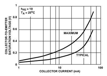
FIGURE 5. COLLECTOR-TO-EMITTER SATURATION VOLTAGE vs COLLECTOR CURRENT
