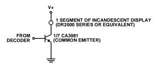
FIGURE 1. SCHEMATIC DIAGRAM SHOWING ONE TRANSISTOR OF THE CA3081 DRIVING ONE SEGMENT OF AN INCANDESCENT DISPLAY
