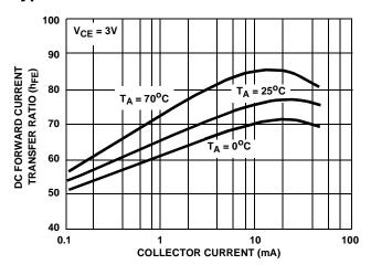
FIGURE 3. DC FORWARD CURRENT TRANSFER RATIO vs COLLECTOR CURRENT
