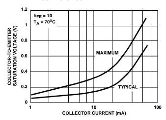
FIGURE 6. COLLECTOR-TO-EMITTER SATURATION VOLTAGE vs COLLECTOR CURRENT
