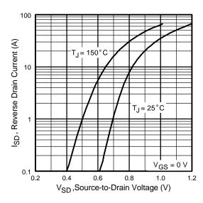
**Fig 8.** Typical Source-Drain Diode Forward Voltage
