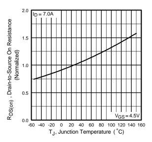
**Fig 5.** Normalized On-Resistance Vs. Temperature
