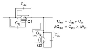
Figure 2: Q<sub>oss</sub> Characteristic
