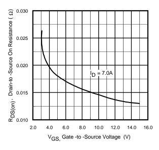
Fig 7. On-Resistance Vs. Gate Voltage
