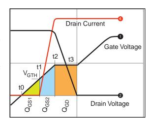
Figure 1: Typical MOSFET switching waveform
