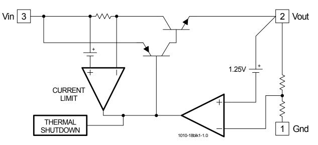
Figure 2 - Simplified block diagram of the IRU1010-18.
