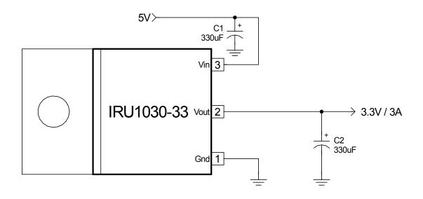
Figure 1 - Typical application of IRU1030-33
