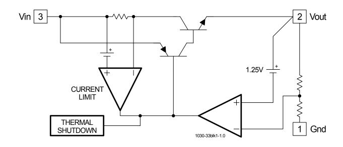
Figure 2 - Simplified block diagram of the IRU1030-33
