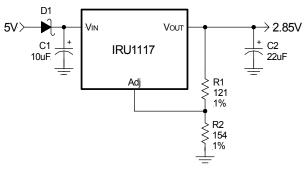
Figure 5 - Final Schematic for half of the GTL+ termination regulator.
