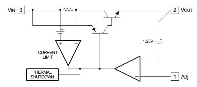
Figure 2 - Simplified block diagram of the IRU1117.
