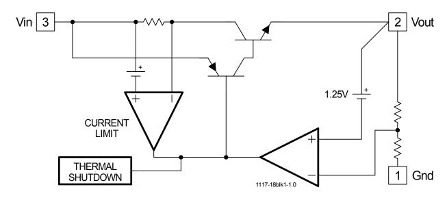
Figure 2 - Simplified block diagram of the IRU1117-18
