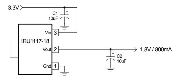
Figure 1 - Typical set-up of the IRU1117-18 in a 3.3V to 1.8V regulator application
