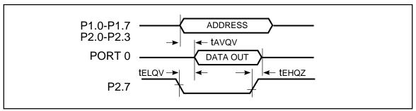
Figure 33. ROM Verification Waveform
