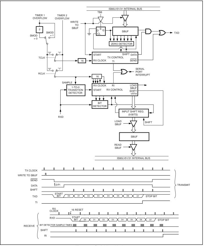
Figure 13. Serial Port Mode 1
