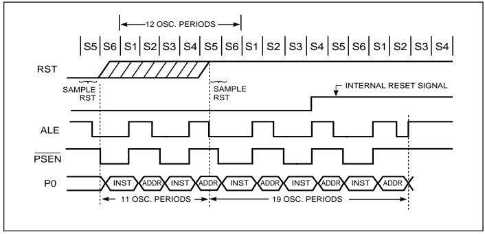
Figure 19. Reset Timing
