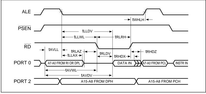
Figure 30. External Data Memory Read Cycle
