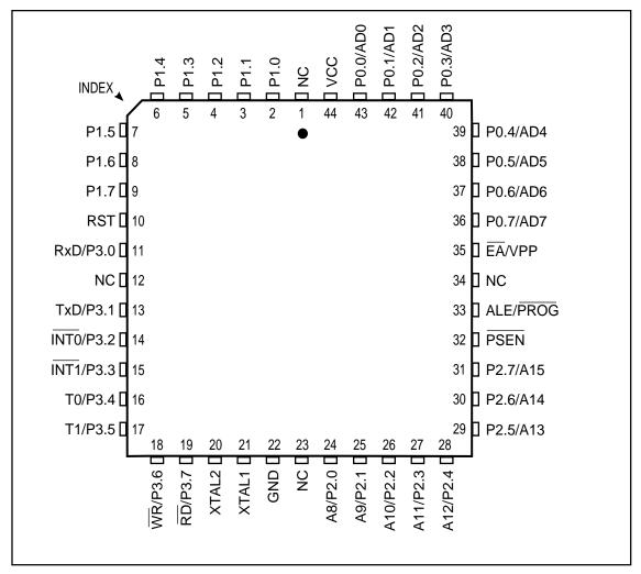
Figure 2. IS80LV51/31 Pin Configuration: 44-pin PLCC
