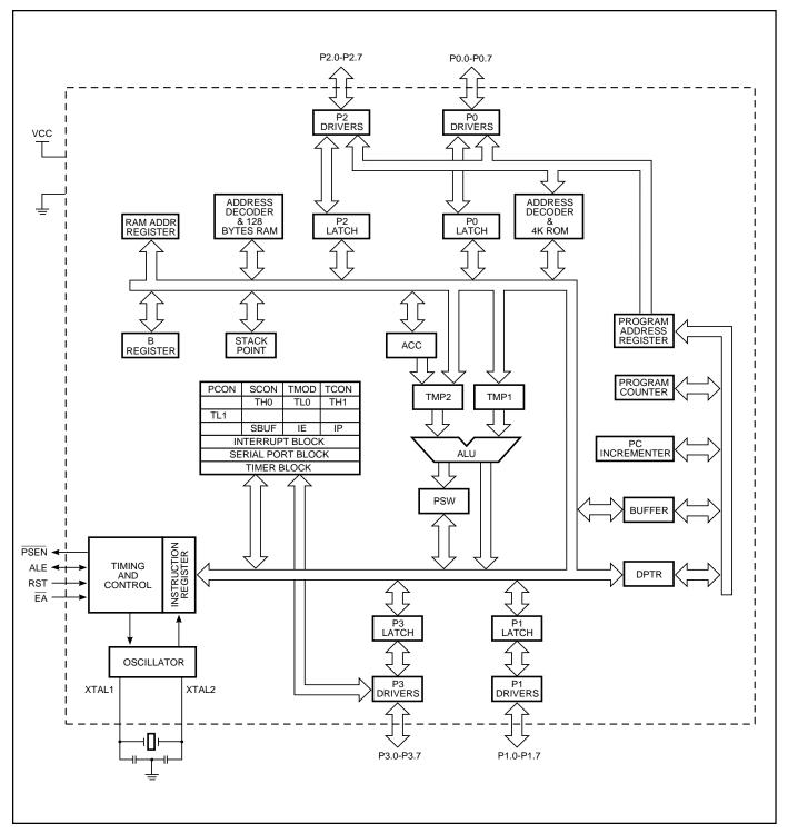
Figure 4. IS80LV51/31 Block Diagram
