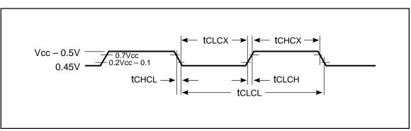
Figure 34. External Clock Drive Waveform
