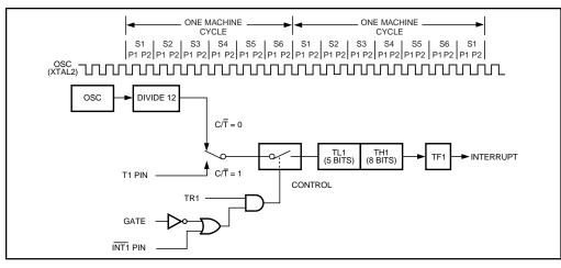
Figure 8. Timer/Counter 1 Mode 0: 13-Bit Counter
