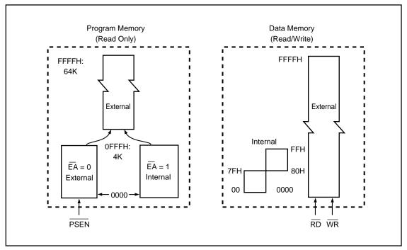
Figure 5. IS80LV51/31 Program and Data Memory Structure
