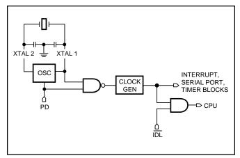
Figure 20. Idle and Power-Down Hardware
