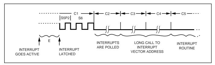
Figure 17. Interrupt Response Timing Diagram
