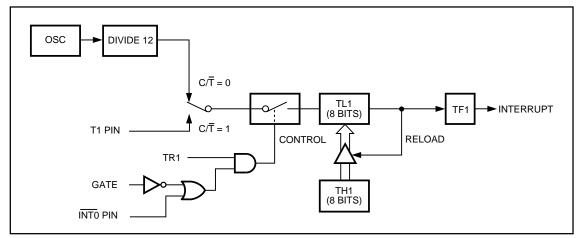
Figure 10. Timer/Counter 1 Mode 2: 8-Bit Auto-Reload
