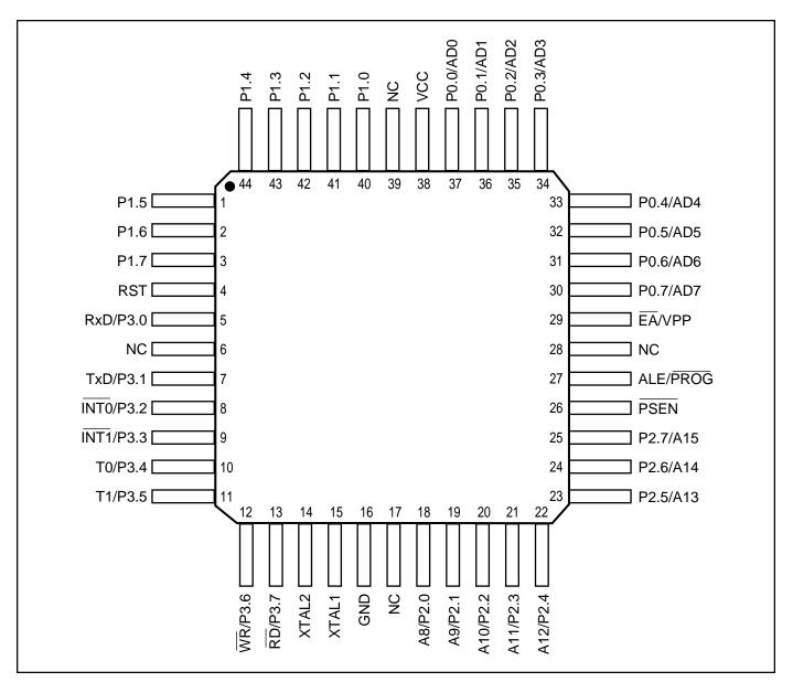
Figure 3. IS80LV51/31 Pin Configuration: 44-pin PQFP
