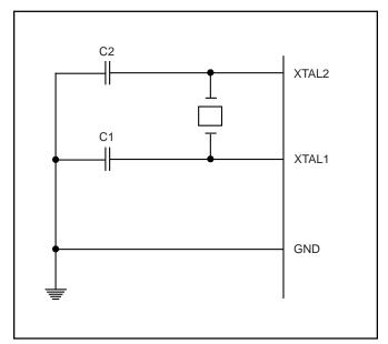
Figure 21. Oscillator Connections
