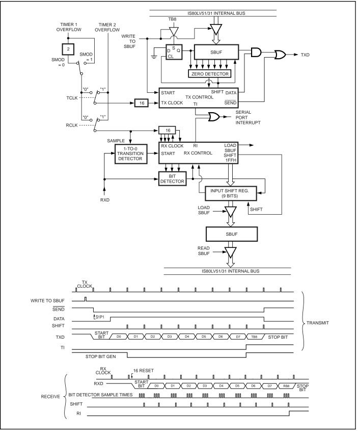
Figure 15. Serial Port Mode 3
