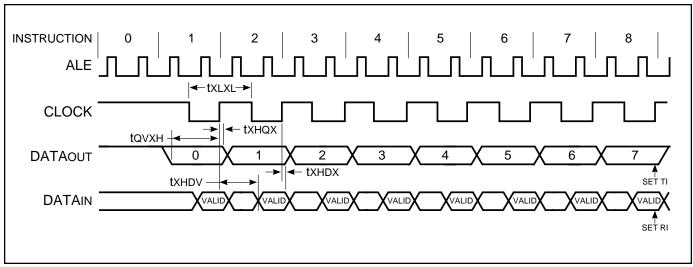
Figure 32. Shift Register Mode Timing Waveform
