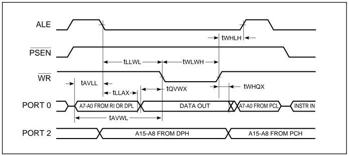
Figure 31. External Data Memory Write Cycle
