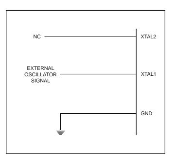
Figure 22. External Clock Drive Configuration
