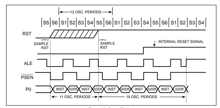
Figure 21. Reset Timing
