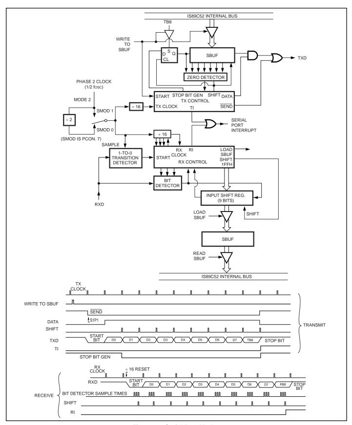
Figure 17. Serial Port Mode 2
