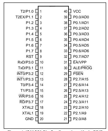
Figure 1. IS89C52 Pin Configuration: 40-pin PDIP
