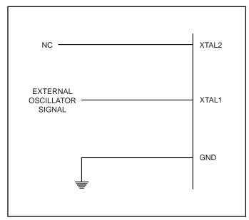
Figure 22. External Clock Drive Configuration
