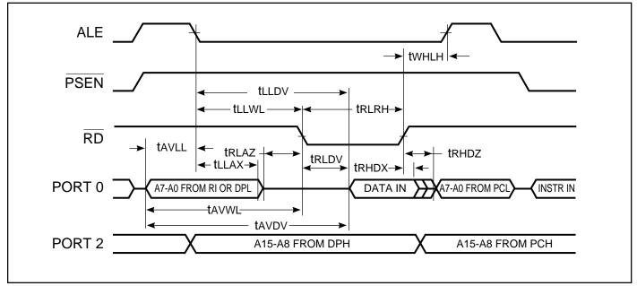
Figure 36. External Data Memory Read Cycle
