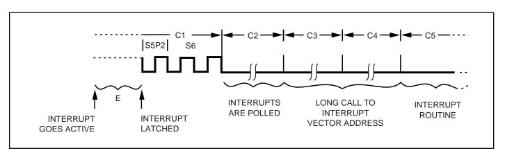
Figure 20. Interrupt Response Timing Diagram
