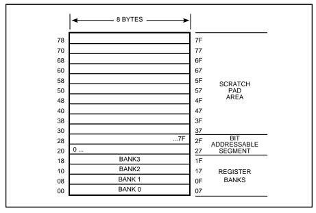
Figure 7. Lower 128 Bytes of Internal RAM
