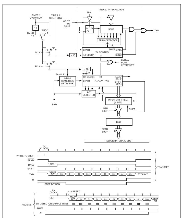
Figure 18. Serial Port Mode 3
