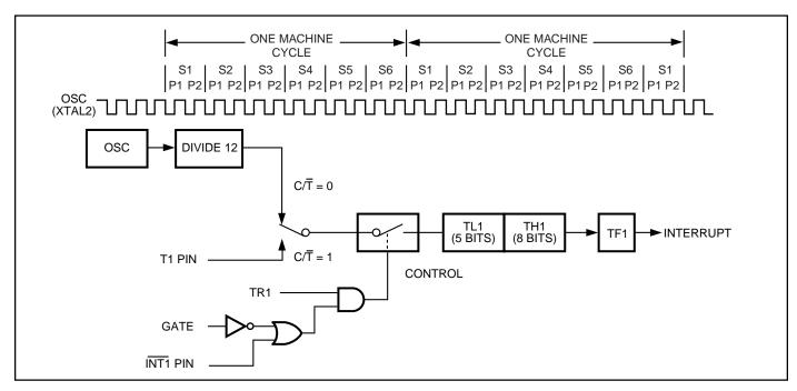
Figure 8. Timer/Counter 1 Mode 0: 13-Bit Counter
