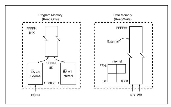
Figure 5. IS89C52 Program and Data Memory Structure
