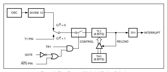
Figure 10. Timer/Counter 1 Mode 2: 8-Bit Auto-Reload
