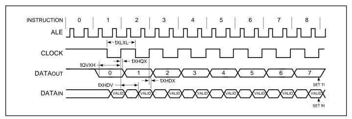
Figure 38. Shift Register Mode Timing Waveform
