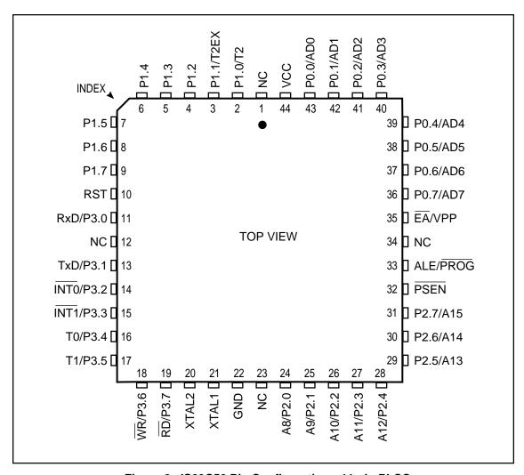
Figure 2. IS89C52 Pin Configuration: 44-pin PLCC
