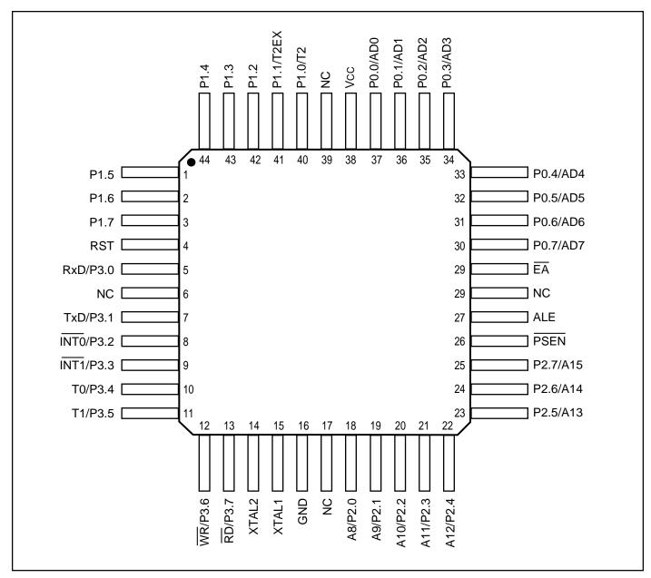
Figure 3. IS89C52 Pin Configuration: 44-pin PQFP
