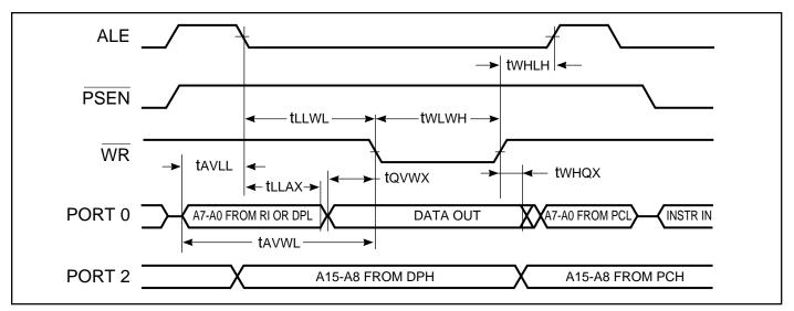
Figure 37. External Data Memory Write Cycle
