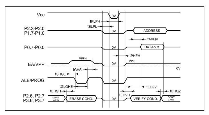
Figure 30. Flash Memory Erase Timing Waveform
