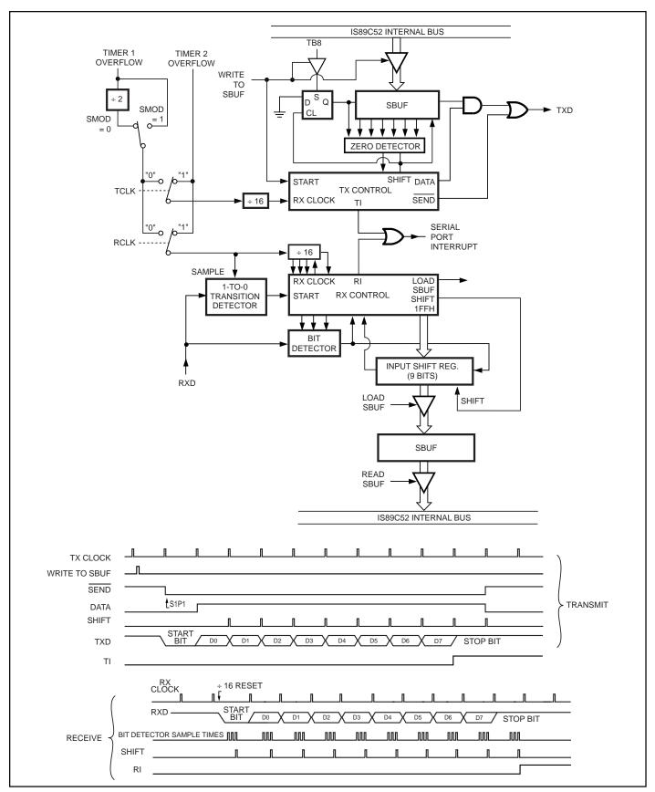
Figure 16. Serial Port Mode 1
