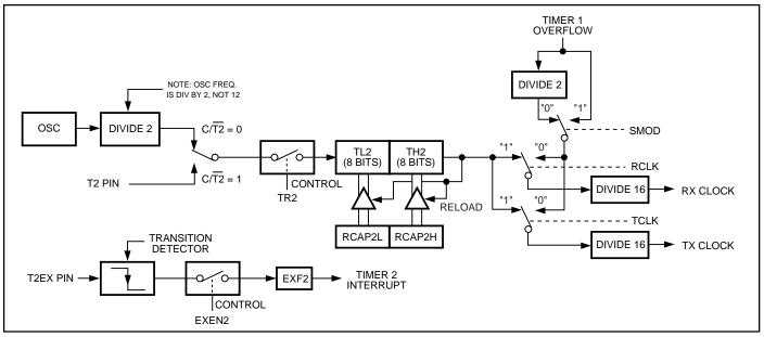
Figure 14. Timer 2 in Baud Rate Generator Mode
