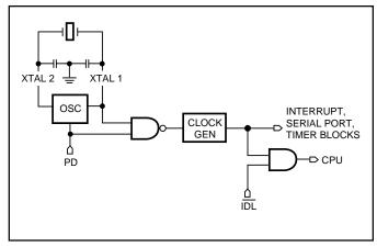
Figure 23. Idle and Power-Down Hardware
