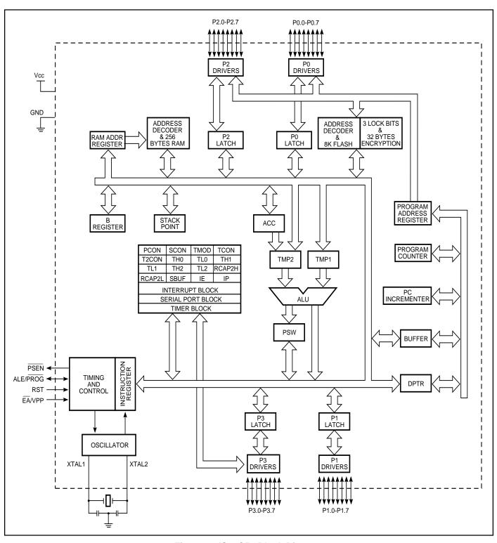
Figure 4. IS89C52 Block Diagram
