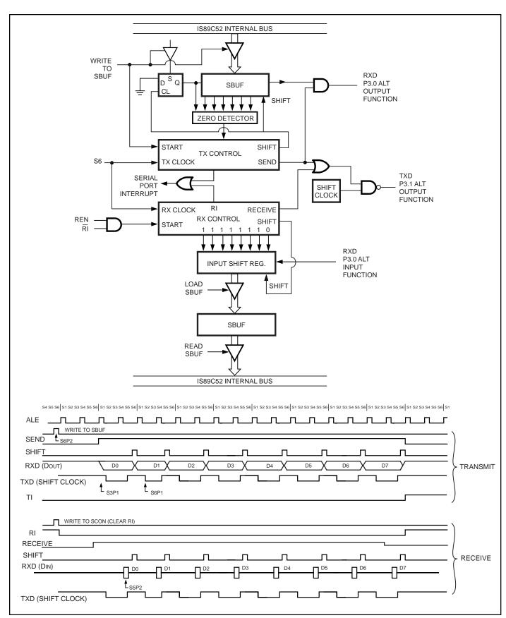
Figure 15. Serial Port Mode 0
