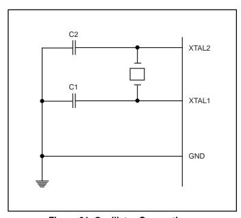
Figure 21. Oscillator Connections
