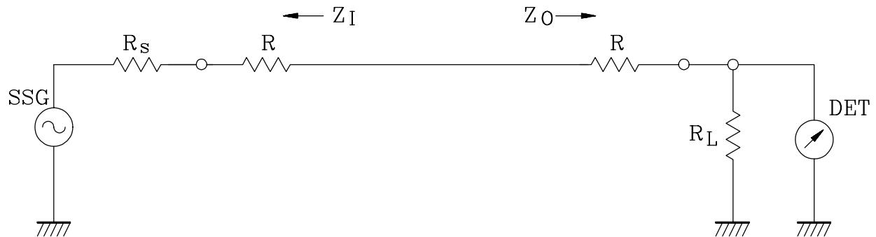
$R_S, R_L : 50\Omega$  (Internal Impedance of Source and Load)
