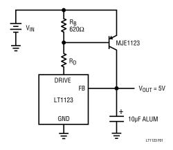
Figure 1. Basic Regulator Circuit
