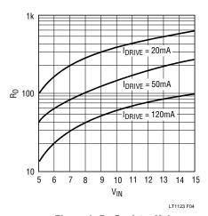
Figure 4. R<sub>D</sub> Resistor Value
