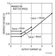
Figure 2. Maximum Dropout Voltage
