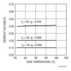
Figure 3. Dropout Voltage vs Temperature
