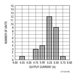
Figure 5. Short Circuit Current for 30 Random Devices
