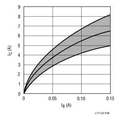
Figure 6. MJE1123 I<sub>C</sub> vs I<sub>B</sub>
