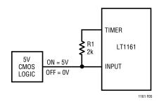
Figure 5. Latch-Off Input Network (Auto-Restart Defeated)
