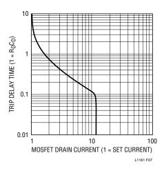
Figure 7. Current Limit Delay Time
