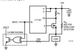
Figure 8. Fault Feedback Using Exclusive-NOR Gate
