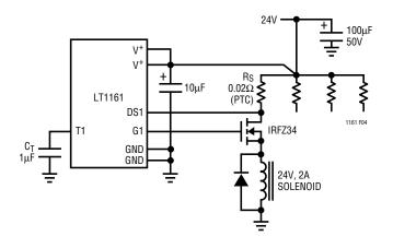
Figure 4. Drain Sense Configuration
