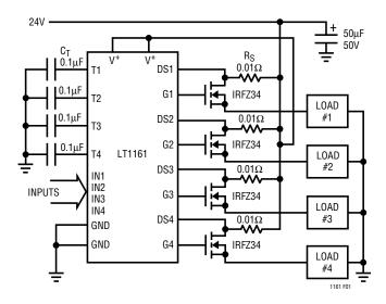
Figure 1. Protected Quad High-Side Switch
