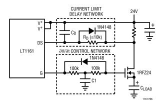
Figure 6. ∂V/∂t Control and Current Limit Delay
