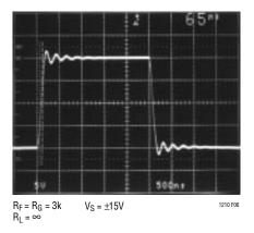
Figure 6. Large-Signal Response, C<sub>L</sub> = 10,000pF
