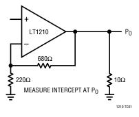
The LT1210 is a current feedback amplifier with high output current drive capability. The device is stable with large capacitive loads and can easily supply the high currents required by capacitive loads. The amplifier will drive low impedance loads such as cables with excellent linearity at high frequencies.
