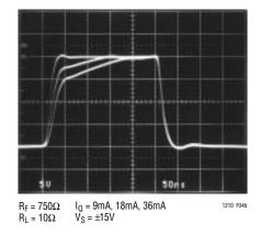
Figure 4b. Large-Signal Response vs  $I_Q$ ,  $A_V = 2$
