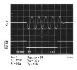
Figure 3. Shutdown Operation
