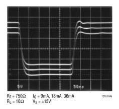
Figure 4a. Large-Signal Response vs  $I_0$ ,  $A_V = -1$
