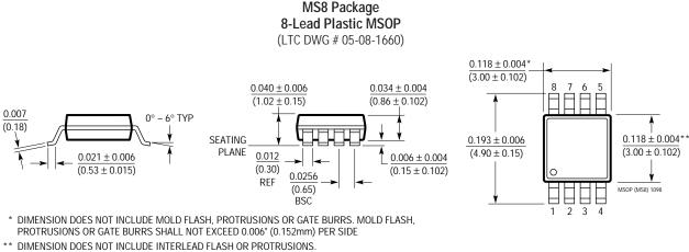
INTERLEAD FLASH OR PROTRUSIONS SHALL NOT EXCEED 0.006" (0.152mm) PER SIDE
