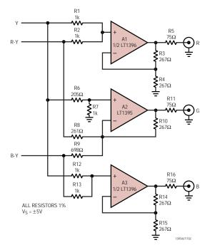
Figure 2. Buffered Color-Difference to RGB Matrix
