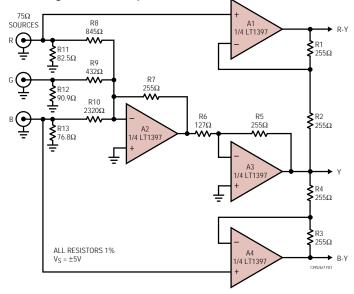
Figure 1. Buffered RGB to Color-Difference Matrix
