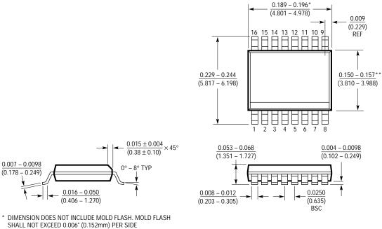
\*\* DIMENSION DOES NOT INCLUDE INTERLEAD FLASH. INTERLEAD FLASH SHALL NOT EXCEED 0.010" (0.254mm) PER SIDE
