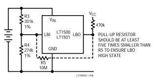
Figure 6. Low Battery Detection
