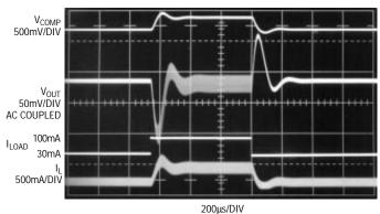
Figure 5. Transient Response of LT1500 with  $R_C$  = 10k,  $C_C$  = 2200pF and  $C_{OUT}$  =15 $\mu F$  Ceramic.  $V_{OUT}$  Disturbance is 100mV
