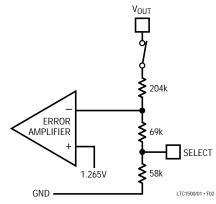
Figure 2. Schematic of Select Pin Function
