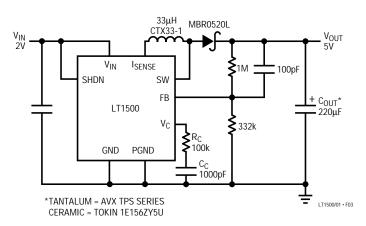
Figure 3. LT1500 2V to 5V Converter
