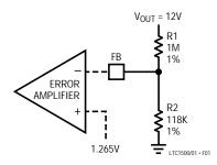
Figure 1. External Voltage Divider
