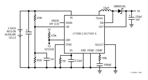
Typical LT1500 (14-Pin) Application, 2-Cell to 5V Converter
