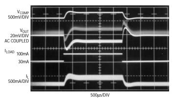
Figure 4. Transient Response of LT1500 with  $R_C = 100k$ ,  $C_C = 1000pF$  and  $C_{OUT} = 220\mu F$ .  $V_{OUT}$  Disturbance is 20mV
