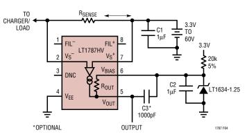
Figure 4. Charge/Discharge Current Monitor on Single Supply with  $V_{BIAS} = 1.25V$
