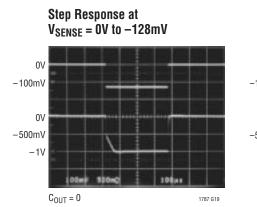
Step Response at V<sub>SENSE</sub> = 0V to -128mV
