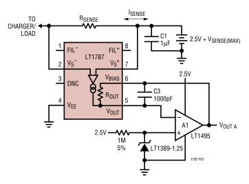
Figure 7. Single Supply 2.5V Bidirectional Operation with External Voltage Reference and I/V Converter
