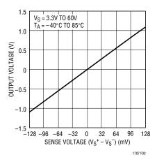
Figure 3. Split Supply Output Voltage
