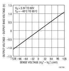
Figure 5. Single Supply Output Voltage with  $V_{BIAS} = 1.25 \text{V}$
