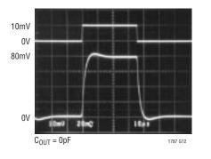
Step Response at  $V_{SENSE} = 0V$  to 128mV
