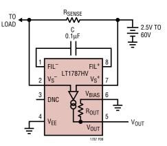
Figure 8. Unidirectional Current Sensing Mode
