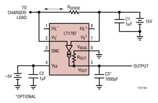
Figure 2. Split Supply Operation
