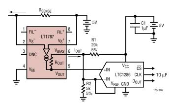
Figure 6. Unidirectional Output into A/D with Fixed Supply at  $\rm V_S^+$
