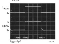
Step Response at V<sub>SENSE</sub> = OV to 128mV
