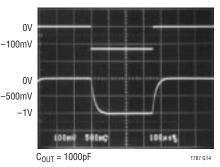
Step Response at  $V_{\text{SENSE}} = -128 \text{mV}$  to 128 mV
