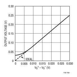
Figure 9. Expanded Scale of Unidirectional Output
