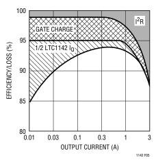
Figure 5. Efficiency Loss
