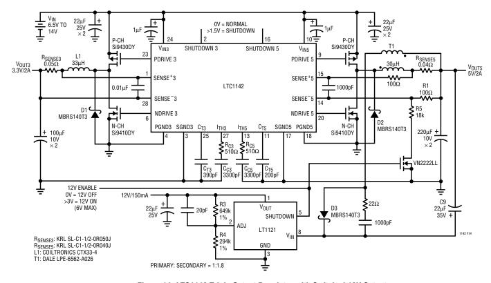
Figure 14. LTC1142 Triple Output Regulator with Switched 12V Output
