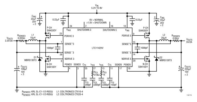
Figure 13. LTC1142HV High Efficiency Regulator with 3.3V/3A and 5V/2A Outputs
