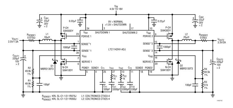
Figure 12. LTC1142HV-ADJ High Efficiency Regulator with 3.3V/2A and 2.5V/1.5A Outputs
