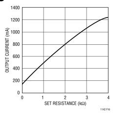
Figure 16. LTC1142HV-ADJ Output Current vs Trickle Charge Set Resistance (R<sub>x</sub>) for the Circuit in Figure 15 Using a  $0.1\Omega$  Current Sense Resistor R<sub>SENSE1</sub>
