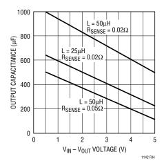
Figure 4. Minimum Value of  $C_{OUT}$
