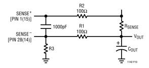
Figure 10. Suppression of Burst Mode Operation
