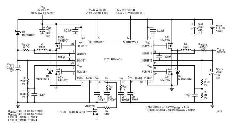
Figure 15. LTC1142HV-ADJ High Efficiency Power Supply Providing 3.3V/2A with Built-In Battery Charger
