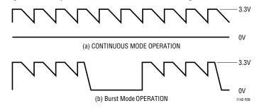
Figure 9. C<sub>T</sub> Waveforms
