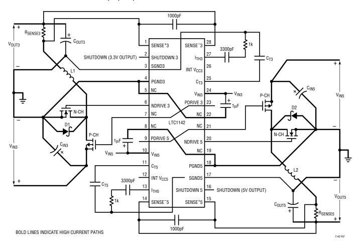
Figure 7. LTC1142 Layout Diagram (see Board Layout Checklist)
