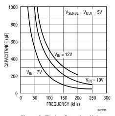
Figure 3. Timing Capacitor Value
