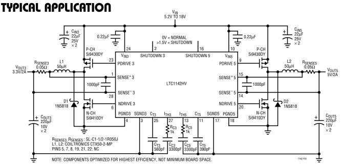
Figure 1. High Efficiency Dual 3.3V, 5V
