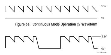
Figure 6b. Burst Mode Operation C<sub>T</sub> Waveform
