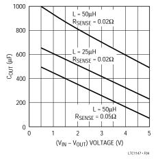
Figure 4. Minimum Value of C<sub>OUT</sub>
