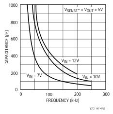
Figure 3. Timing Capacitor Value
