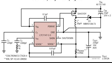
3.3V/2A Output High Efficiency Regulator
