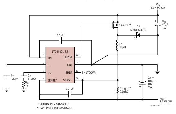
3.3V Low Dropout High Efficiency Regulator
