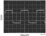
BESSEL RATIO = 140:1  $f_{CLK} = 700 kHz$  $f_C = 5kHz$  $V_S = \pm 7.5 V$
