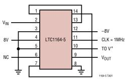
WIDEBAND NOISE = 110  $\mu V_{RMS}$  Thd in Passband < 0.02% at  $V_{IN}$  = 2  $V_{RMS}$
