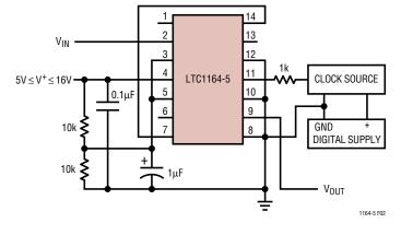
Figure 2. Single Supply Operation for  $f_{CLK}/f_{CUTOFF} = 100:1$
