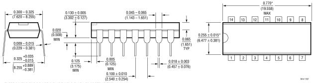
\*THESE DIMENSIONS DO NOT INCLUDE MOLD FLASH OR PROTRUSIONS. MOLD FLASH OR PROTRUSIONS SHALL NOT EXCEED 0.010 INCH (0.254mm)
