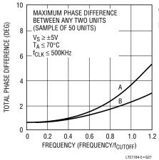
A. BUTTERWORTH  $(f_{CLK}/f_{CUTOFF} = 100:1 \text{ OR } 50:1)$ B. BESSEL ( $f_{CLK}/f_{CUTOFF} = 140:1$ )
