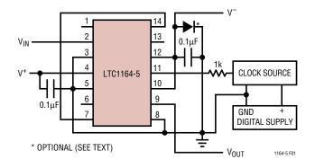
Figure 1. Dual Supply Operation for  $f_{CLK}/f_{CUTOFF} = 100:1$
