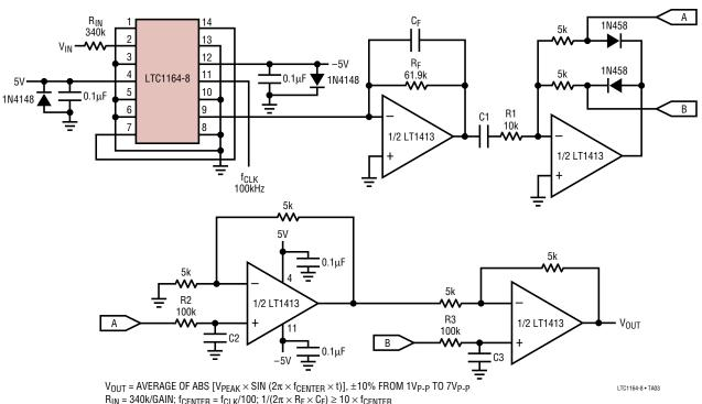
$R_{IN} = 340 \text{k/GAIN}; \ f_{CENTER} = f_{CLK}/100; \ 1/(2\pi \times R_F \times C_F) \geq 10 \times f_{CENTER}$
