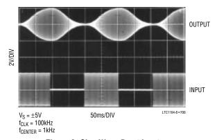
Figure 6. Sine Wave Burst Input
