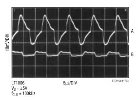
Figure 4. Clock Feedthrough at the Output of External Op Amp A. With No Capacitor Across Feedback Resistor  $R_F$  B. With Capacitor  $C_F$  Across Feedback Resistor  $R_F$   $1/(2\pi \bullet R_F \bullet C_F) = 10 \bullet f_{CENTER}$
