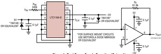
Figure 1. Dual Power Supply Operation (Gain = 1)
