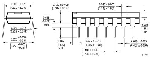
\*THESE DIMENSIONS DO NOT INCLUDE MOLD FLASH OR PROTRUSIONS. MOLD FLASH OR PROTRUSIONS SHALL NOT EXCEED 0.010 INCH (0.254mm).
