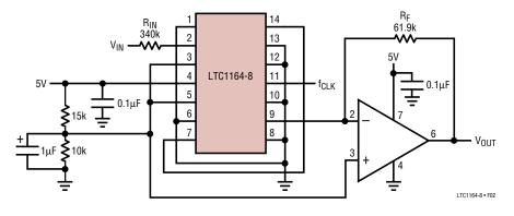
Figure 2. Single Power Supply Operation (Gain = 1)
