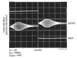
Figure 5. Square Wave Input  $(\pm 2.5V)$
